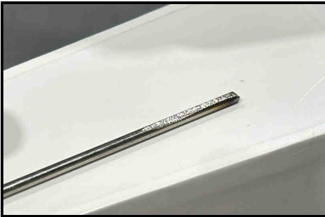
Be sure to install the flat portion of the tiller wire into the tailwheel swivel mount. Apply Loctite to the set screw before tightening.
