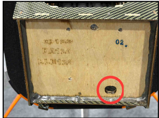
If you plan to install the throttle servo inside the motor box, drill a hole for the linkage as shown.
