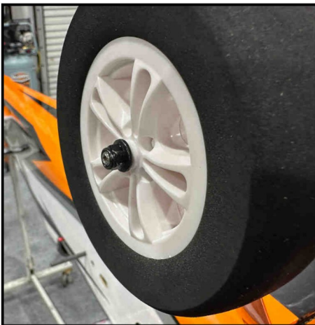
Thread the collar nut onto the axle and tighten it securely, taking care not to overtighten.
