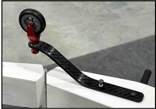
The tailwheel is installed using two bolts. Apply blue Loctite to the bolts before tightening.
