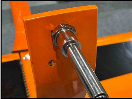
Align the axle so that the hex portion is vertical. This orientation ensures the wheel pant can be installed correctly.
