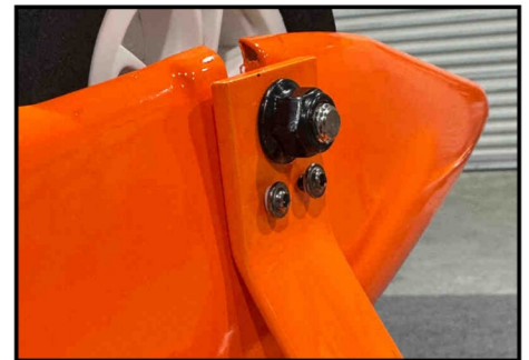
The wheel pants are installed using two M3 bolts. Apply blue Loctite to the bolts before installation.
