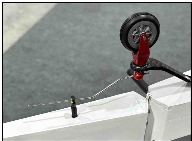
Bend the tiller wire so it aligns with the opening of the ball link. Applying heat while the wire is off and away from the aircraft is a simple and effective method to achieve the correct bend.
