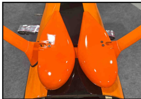
The wheel pants are installed using two M3 bolts. Apply blue Loctite to the bolts before installation.
