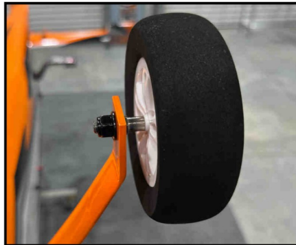
Locate the wheel and tire assembly and slide it onto the axle.
