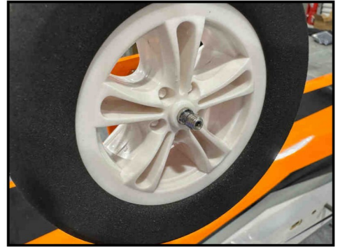
Apply blue Loctite to the threaded end of the axle before installing the collar nut.
