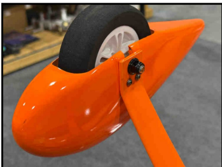
Thread the collar nut onto the axle and tighten it securely, taking care not to overtighten.
