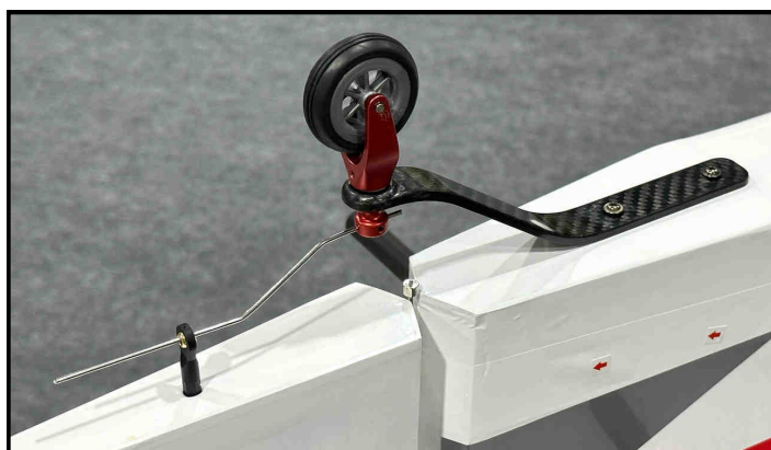
Tailwheel assembly complete. Verify that the rudder moves freely and achieves full deflection in both directions.
